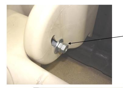
Tighten the two jam nuts securely against each other so they do not come loose. Loctite may also be used but is not required. The  $\frac{1}{2} \ge 9$   $\frac{1}{2}$ " bolt should remain slightly loose so it is free to move in the slot.
