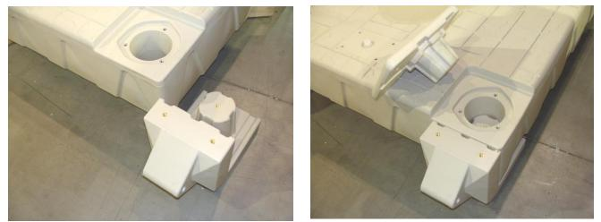
**2.** Insert top connection piece into post hole and secure to bottom connection using the  $3/8 \ge 2$  bolts, lock washers and flat washers in three locations. Lock washers will be on top of the flat washers. Repeat on the other side.
