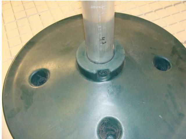
2. Insert the umbrella sleeve into the molded hole in the table top. (See Page 3. if you do not have this molded hole in the table top.) Be sure to align the holes in the sleeve with the bolt hole in the bottom of the table top. This is the same bolt hole as shown in step 1. Do not insert the bolt yet.
