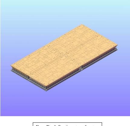
Four Dock Sections together to form 10ft x 20 ft section
