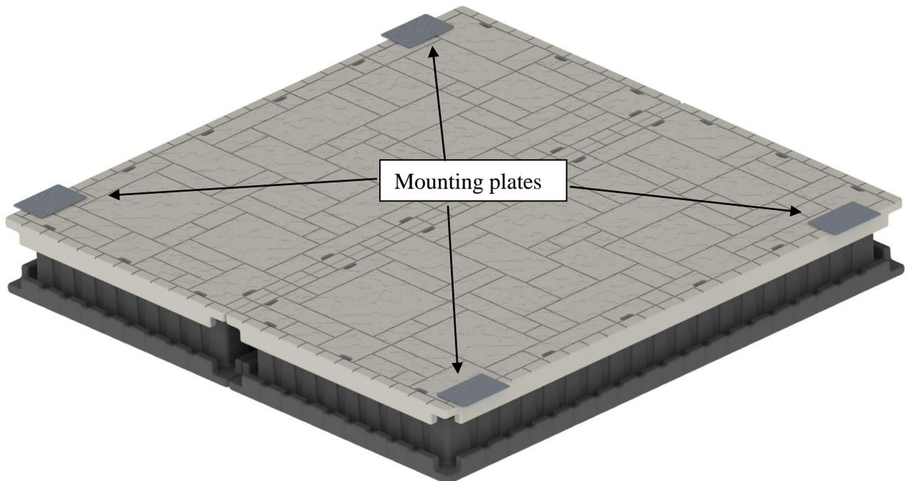
4. Once all of the mounting plates are in place and the Pergola is aligned with the plates then the holes to mount the Pergola to the plates can be marked and drilled. Fasten the plates to the Pergola with either a flat head tapered bolt or a truss head bolt inserted from the bottom of the plate. Using one of these types will avoid damaging the dock surface.
